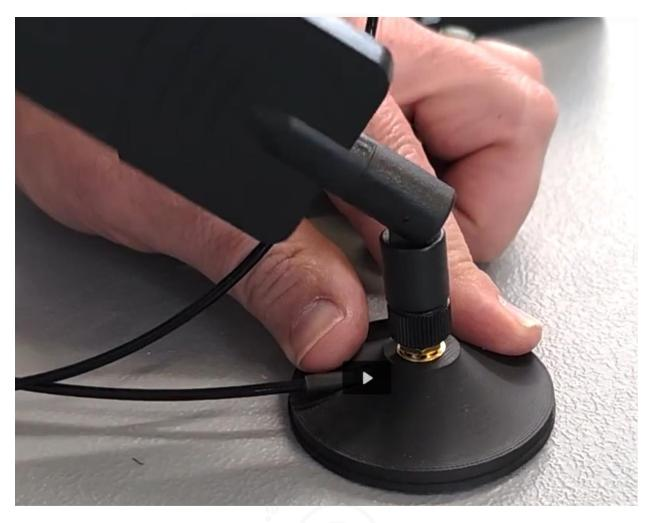
Once the antenna is properly adjusted to its proper position, it can be rotated 180 degrees in either direction at the SMA connector joint to achieve the overall desired orientation.
