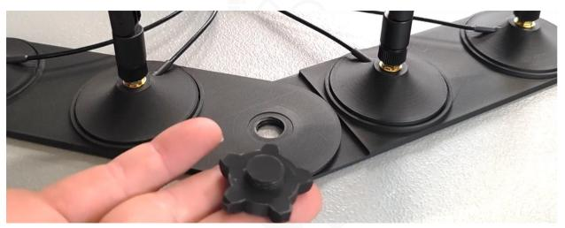
Make certain to gently align the threads of the pivot bolt with the base receiver threads, ensuring not to cross-thread them.
