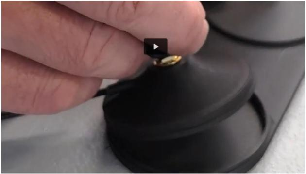
Press the round antenna base into the receiver cup evenly and firmly until it is secured in place inside the receiver cup of the Boomerang™ antenna base.
