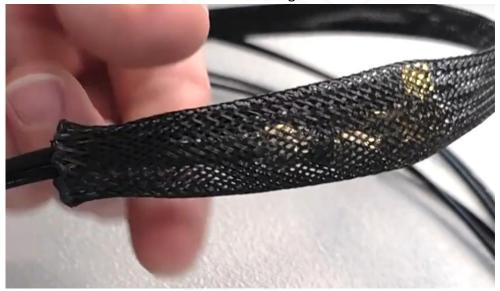
Reverse the ends of the loom by pressing it back into itself:
