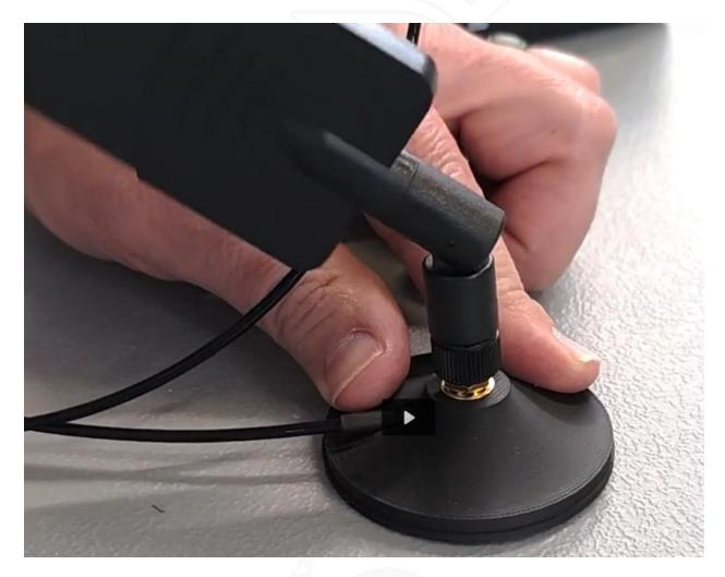
Once the antenna is properly adjusted to its proper position, it can be rotated 180 degrees in either direction at the SMA connector joint to achieve the overall desired orientation.
