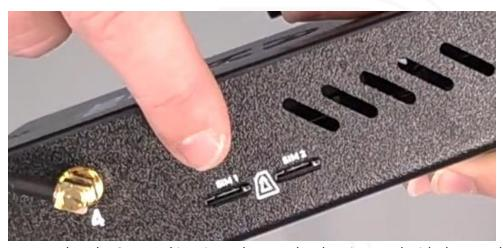
Be sure that the SIM card is oriented correctly when inserted with the metal contacts in the downward position.
